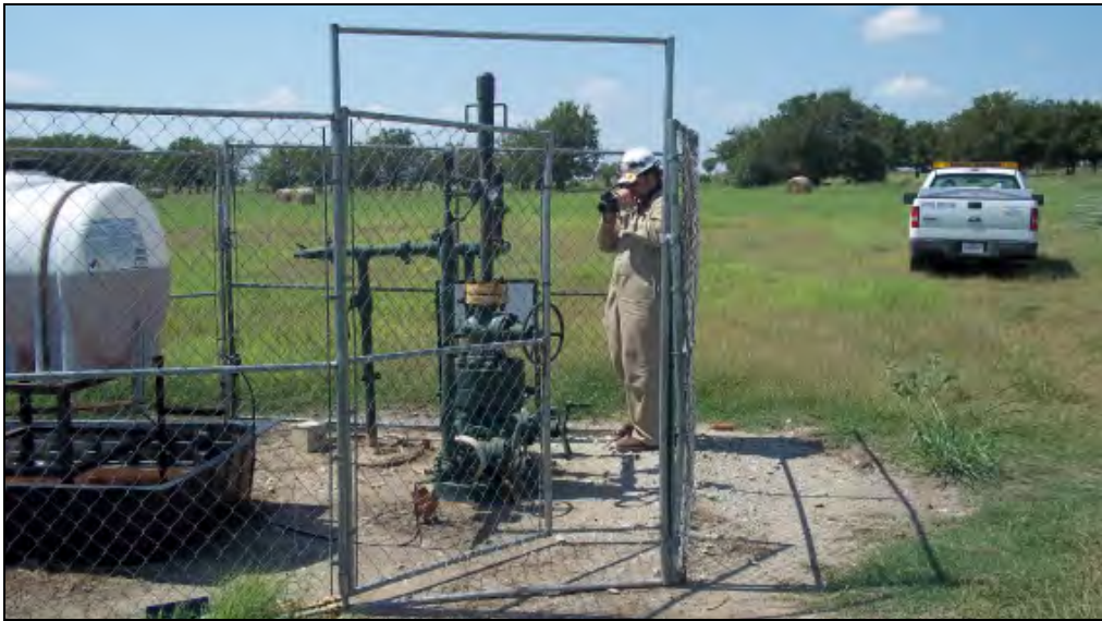
Figure 3.2-1. IR Camera Imaging at a Well Site
