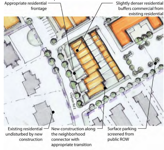
Transition Zone – Recommended Block and Building Layout
