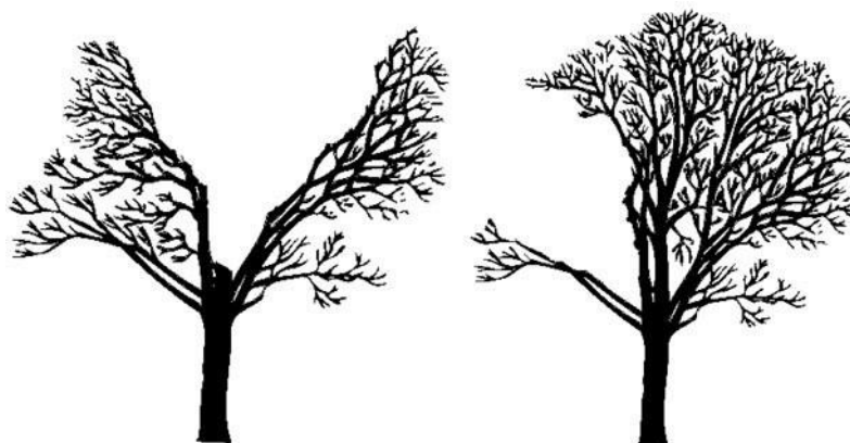
Figure 112. Examples of trees directionally pruned for clearance from power lines
