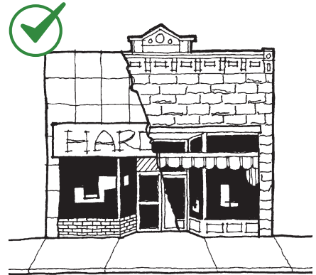
Removal of covering material exposes historic building fabric.
