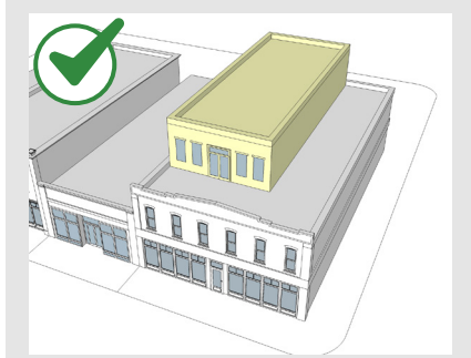
The addition is set back from both the front and side walls.
