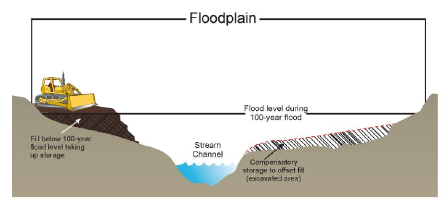
Village of Winnetka, IL, "Floodplain Construction": "Compensatory storage must equal at least 1.1 times the volume of flood storage lost below the Base Flood Elevation (BFE)." Cut or excavate existing ground to mitigate fill in the floodplain.
