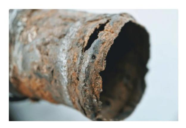
To address frequent main breaks, Fort Worth Water management has committed to replacing a minimum of 20 miles of cast iron pipe every year.
